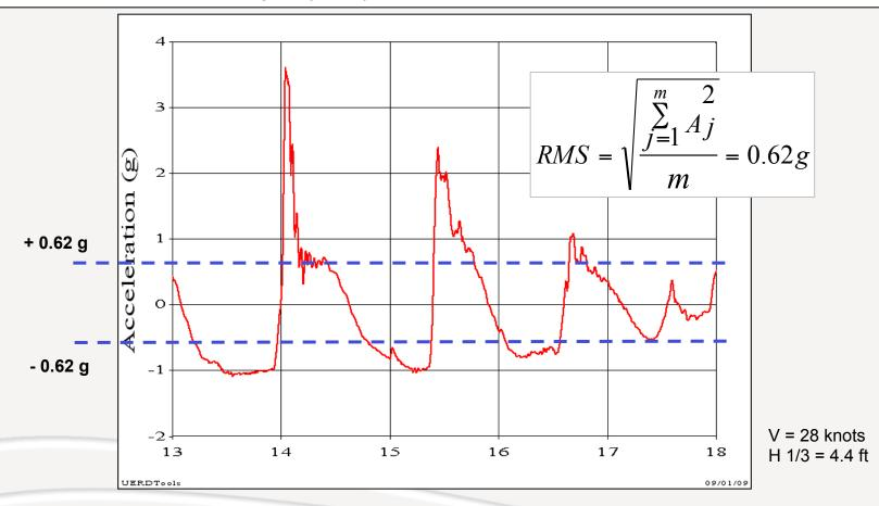
It is therefore recommended that a vertical threshold equal to the RMS acceleration be used
