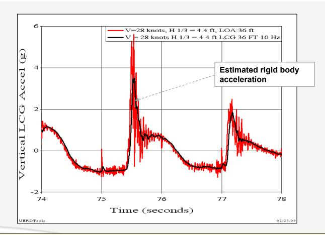
It is therefore recommended that a 10 Hz low pass filter be considered for post-trial data processing to estimate craft rigid body accelerations.
