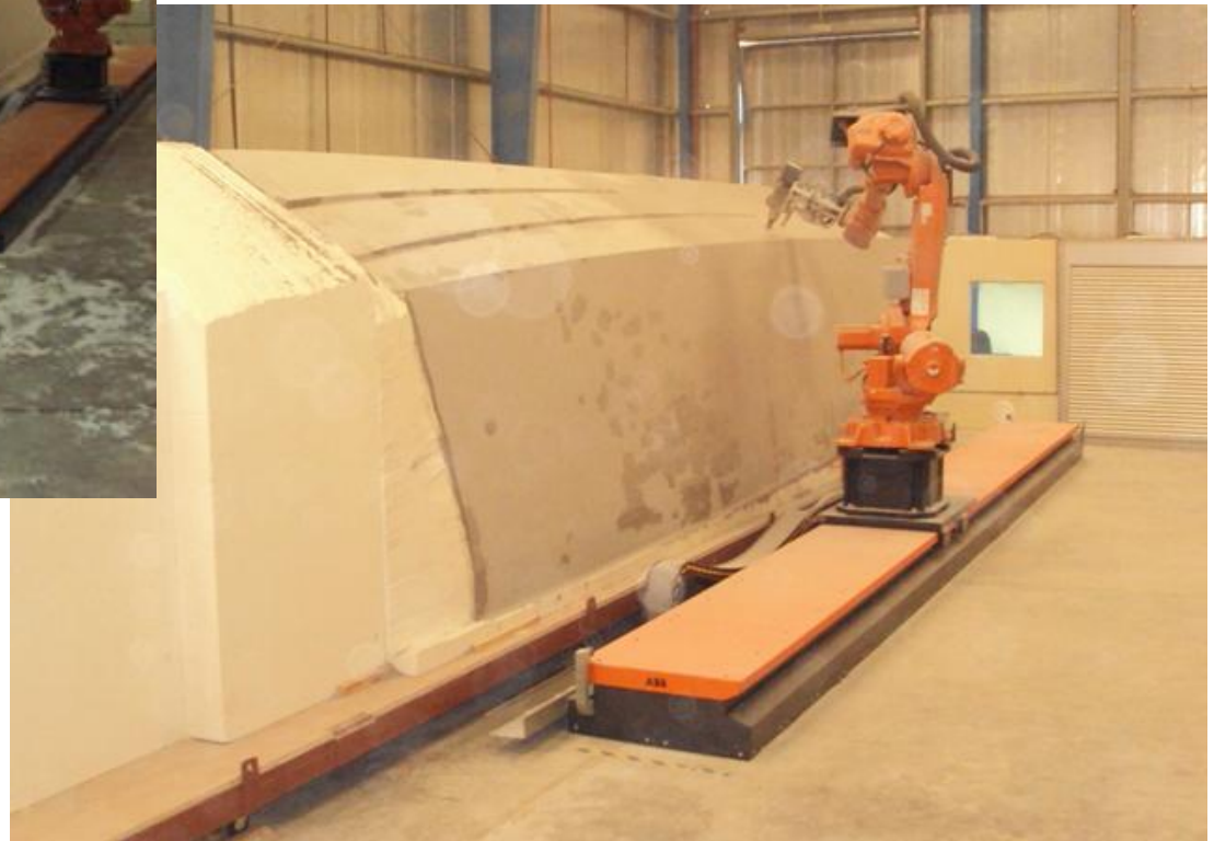
Some of SM16 construction snapshots: CNC-cutting of hull plug
