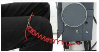
Small, open powerboats should be fitted with a kill cord, which if used correctly, will stop the engine if the driver becomes dislodged from the helm position.
