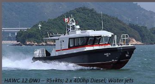
HAWC 12 DWJ – 35+kts; 2 x 400hp Diesel; Water jets
