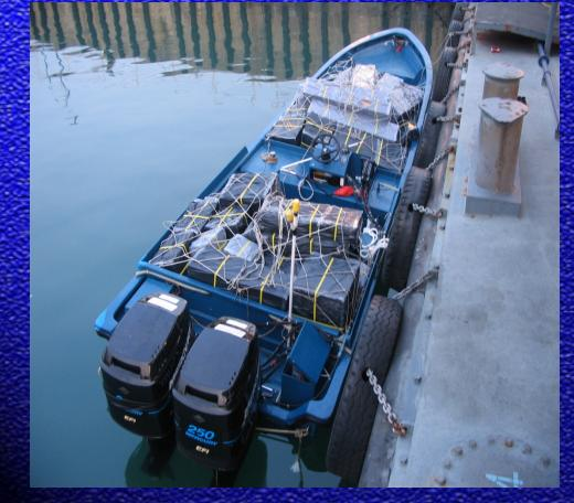
Chung Feis Speed: 45-65Kts Multiple outboard engines Re-inforced Bow
