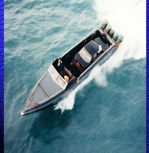
Daai Feis Speed: 35-45Kts Multiple outboard engines Steel Claded Cockpit Re-inforced Bow (ramming)
