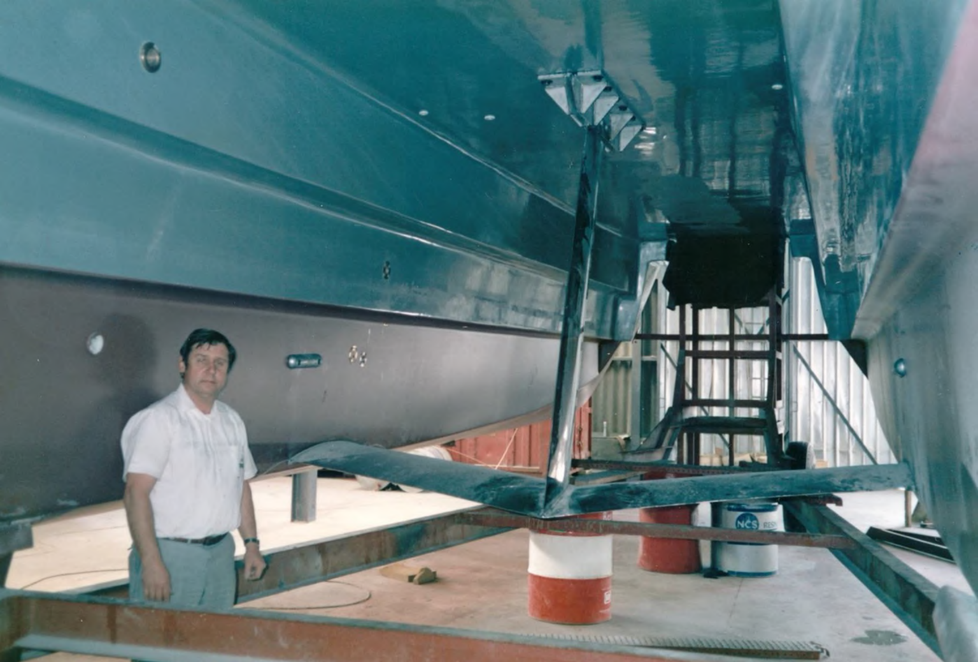
Fig. 11: Foil system of 20m S.A. Navy Offshore Patrol Hysucat
