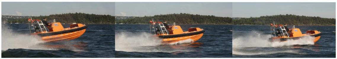
Sequence of 8 pictures per second at 38 knots speed in moderate chop and approx 5m/s wind
