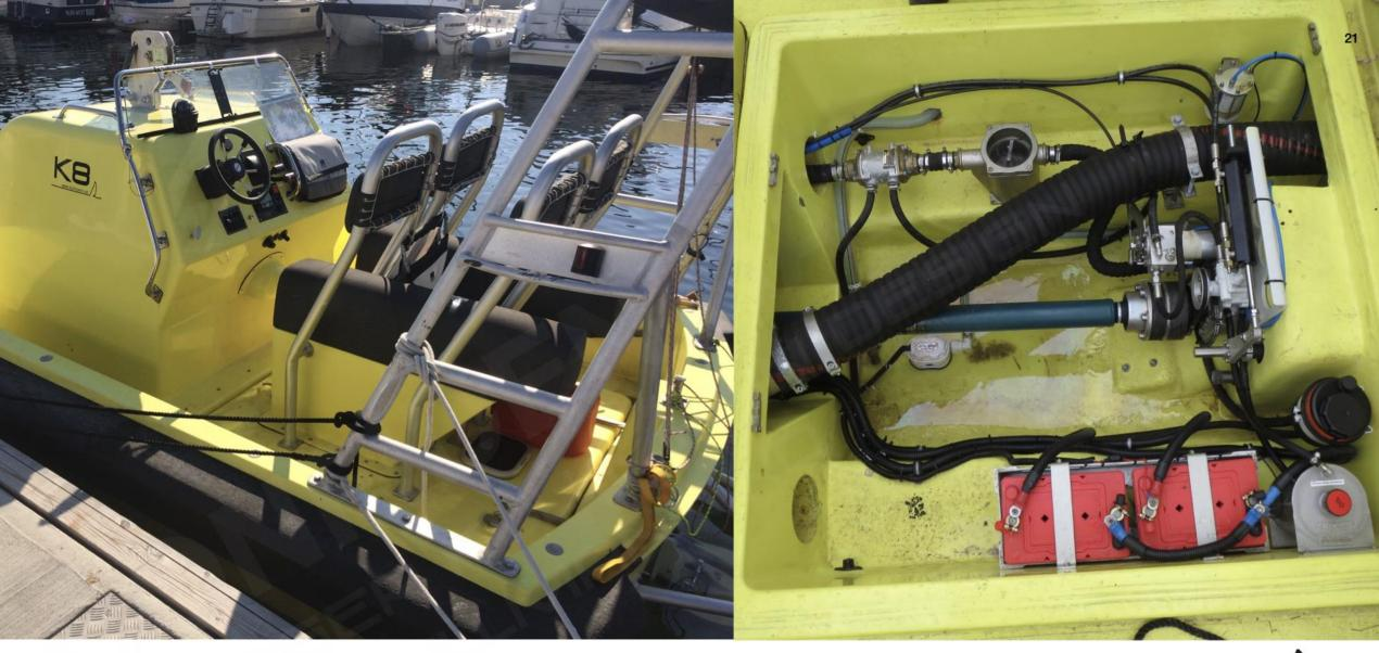
Seats bolted to aft hatch. Hatch raised above deck. Hatch hinged aft, opens to 95 degrees. Access to waterjet, steering, batteries, filters, shaft and so on.
