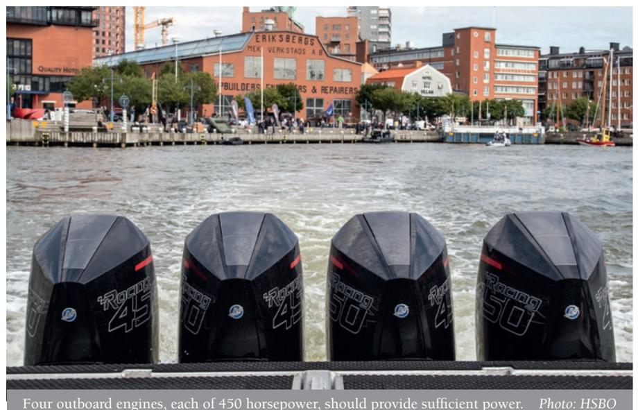
Four outboard engines, each of 450 horsepower, should provide sufficient power. Photo: HSBO
